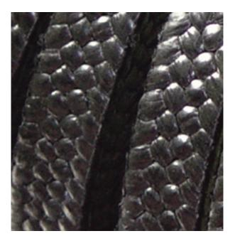
AIGI 16 is braided from PTFE yarn and then coated with high purity graphite, AIGI 16 is a dense braid which ensures excellent leakage control, less lubricant migration, less frictional heat build up and excellent heat dissi- pation for longer life. As a low-friction packing, AIGI 16 is used widely in general service pump applications, specially for ammonia pump, plunger and reciprocating pump.
