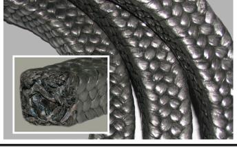
AIGI 22 is made from a high strength, high purity carbon fiber with only minor quantities of braiding sizings added giving the finished packing great temperature and pressure resistance. It is designed for use in high temperature valves and pumps against steam, hot water, solvents, acids and alkalies especially in Power Stations
